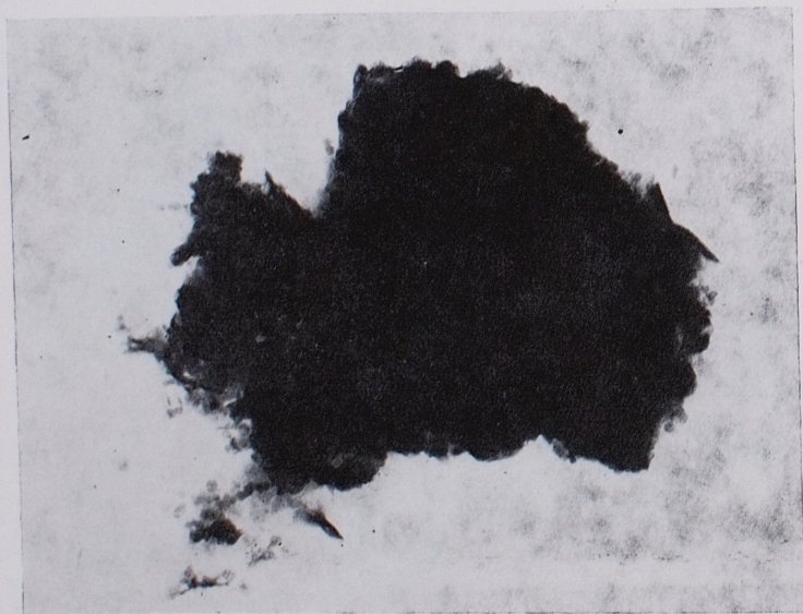
Phot. 4. Electron micrograph of fluorinated montmorillonite ( M-4 sample). \times 40\,000
