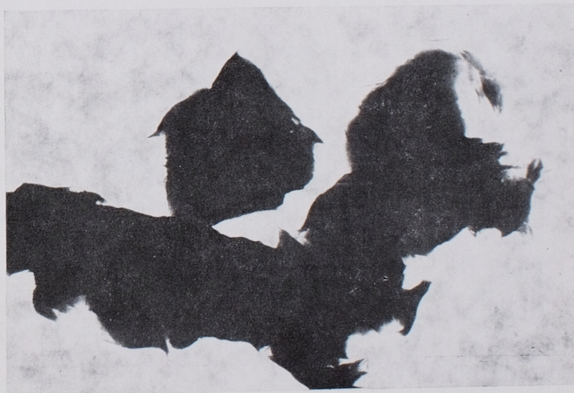
Phot. 2. Electron micrograph of untreated montmorillonite from Chmielnik. \times 20\ 000
